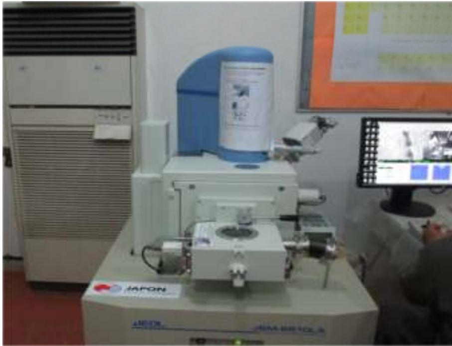
*Figure III. 13* Appareil MEB JEOL (JSM-6610LA) LMESM, USTO-MB.
