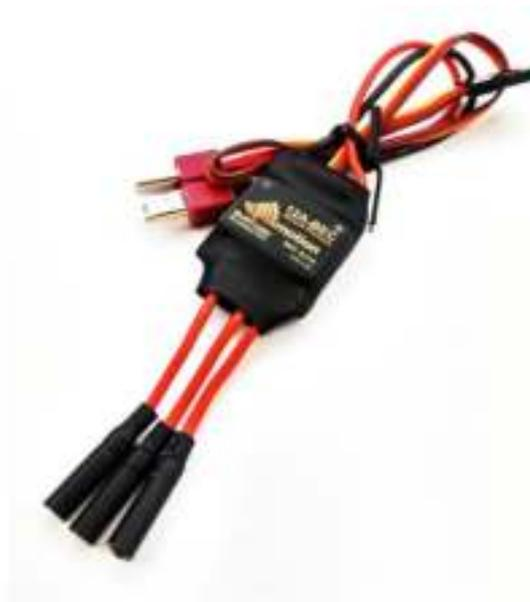
FIGURE 3.10 – Lynxmotion 12A Multicopter ESC.
