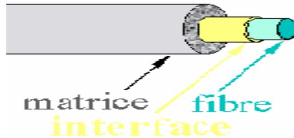
*Figure II.1. Interface fibre/ matrice*
