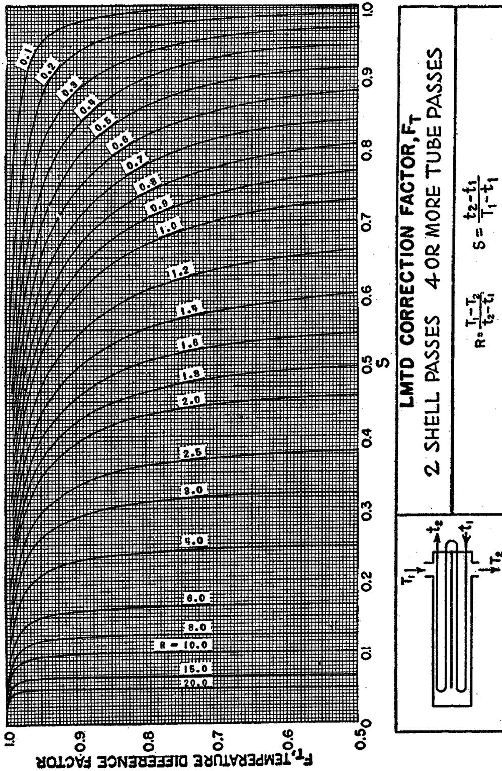
Fig. 19. LMTD correction factors for 2-4 exchangers. (Standards of Tubular Exchanger Manufacturers Association 2d ed., New York, 1949.)
