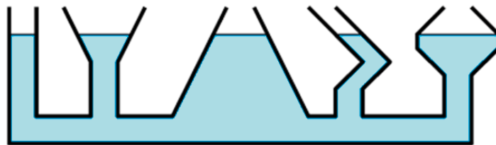
Figure II.6 : Principe de vases communicants.
