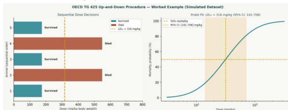
Figure 2.E1. OECD TG 425 Up-and-Down Procedure worked example. Left: sequential dose-outcome pattern for 5 animals (S=survived, D=died) with starting dose 175 mg/kg and 3.16-fold progression. Right: probit dose-response curve fitted to the binary data, with maximum likelihood LD 50 estimate of 316 mg/kg (95% CI: 178–562 mg/kg, shaded).
