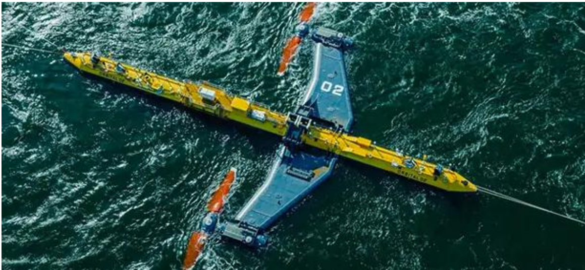
Fig. 3.4 - Orbital Marine Power's floating O2 hydrokinetic (2 MW) during deployment in Scotland [7].
