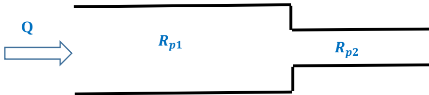
Figure 34: Series arrangement of two pipes.
