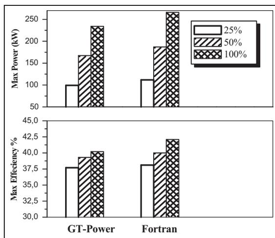
**Figure 14.** Maximum power and maximum efficiency for different fuel masses injected: 25%, 50%, and 100%.
