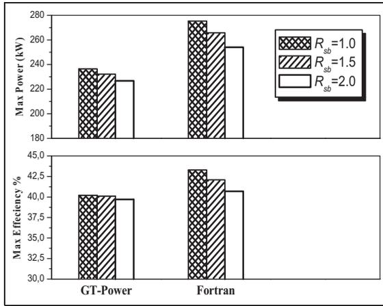
**Figure 7.** Maximum power and maximum efficiency for different stroke–bore ratios:  $R_{sb} = 1.0, 1.5,$  and  $2.0$ .
