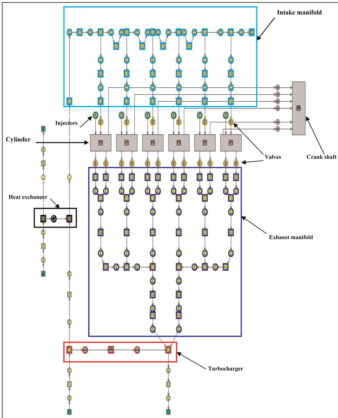
**Figure 3.** Developed model in the commercial engine simulation code GT-Power.<sup>15</sup>
