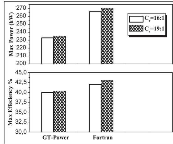
**Figure 5.** Maximum power and maximum efficiency for different compression ratios.
