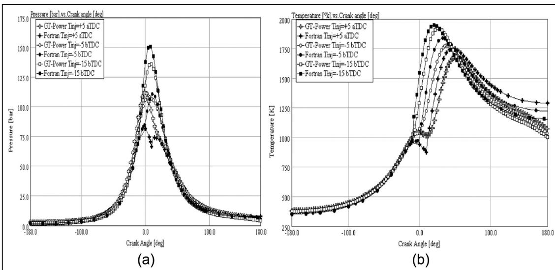
**Figure 12.** (a) Injection timing influence on gas pressure versus crankshaft for 100% load:  $D_{cyl} = 120$  mm;  $c_r = 16:1$ ;  $T_{wall} = 450$  K;  $R_{sb} = 1.5$ ;  $N = 1400$  rpm. (b) Injection timing influence on gas temperature versus crankshaft for 100% load:  $D_{cyl} = 120$  mm;  $c_r = 16:1$ ;  $T_{wall} = 450$  K;  $R_{sb} = 1.5$ ,  $N = 1400$  rpm.
