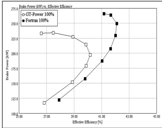
**Figure 4.** Brake power versus effective efficiency for full load:  $T_{inj} = 15^\circ$  bTDC;  $D_{cyl} = 120$  mm;  $c_r = 16:1$ ;  $T_{wall} = 450$  K;  $R_{sb} = 1.5$ .
