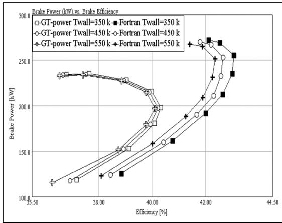
**Figure 10.** Wall temperature influence for 100% load:  $T_{inj} = 15^\circ$  bTDC;  $D_{cyl} = 120$  mm;  $c_r = 16:1$ ;  $R_{sb} = 1.5$ .
