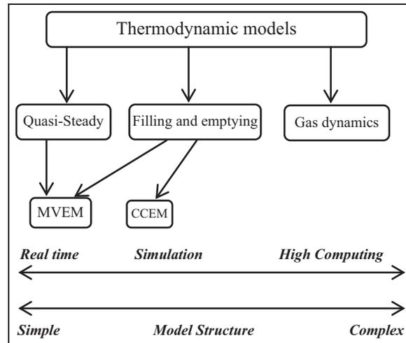
**Figure 1.** Basic classification of thermodynamic models of internal combustion engines. CCEM: cylinder-to-cylinder engine model; MVEM: mean value engine model.
