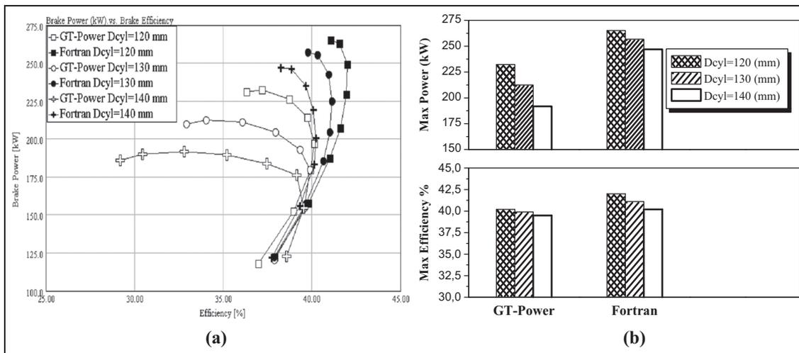
**Figure 6.** (a) Cylinder bore influence for 100% load:  $T_{inj} = 15^\circ$  bTDC;  $D_{cyl} = 120$  mm;  $c_r = 16:1$ . (b) Maximum power and maximum efficiency for different cylinder bore:  $D_{cyl} = 120, 130,$  and  $140$  mm.
