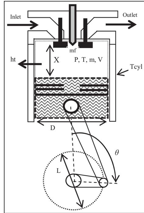
**Figure 2.** Cylinder scheme and its variables. P: pressure, T: temperature, m: mass, V: volume.
