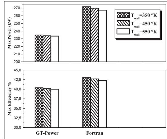
**Figure 9.** Maximum power and maximum efficiency for different cylinder wall temperatures.
