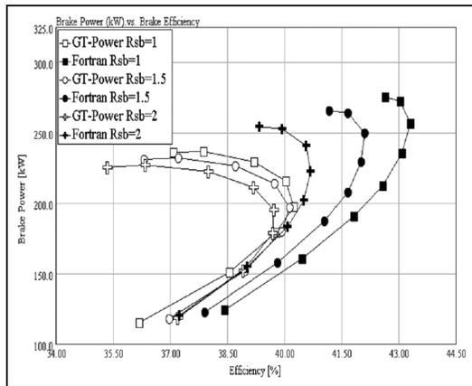
**Figure 8.** Influence of the stroke–bore ratio for 100% load:  $T_{inj} = 15^\circ$  bTDC;  $v_{cyl} = 2.0$  L;  $c_r = 16:1$ ;  $T_{wall} = 450$  K.
