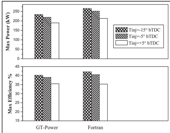
**Figure 11.** Maximum power and maximum efficiency for different injection timings.
