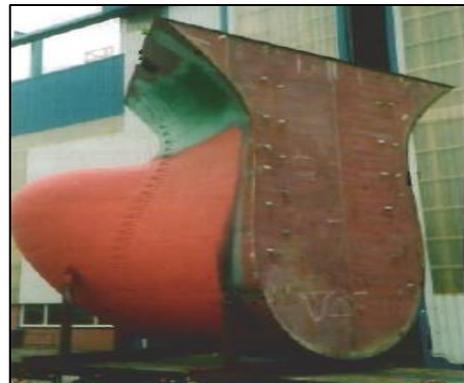
Figure VIII.3. Construction de bulbe.
