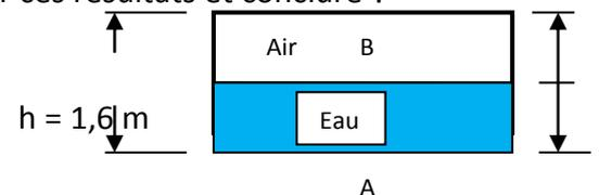
$$\Delta P_{AB} = \rho_{\text{eau}} g (h_A - h_B) = \rho_{\text{eau}} g h/2 \quad \text{soit} \quad \Delta P_{AB} = 10^3 \cdot 9.81 \cdot 0.8 = 7\,848 \text{ Pa}$$
