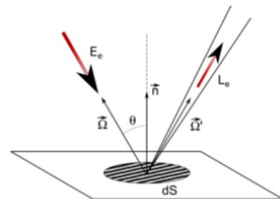
$$\mu \frac{dI(\tau, \mu)}{d\tau} = -I(\tau, \mu) + \frac{1}{2} \int_{-1}^1 p(\mu, \mu') I(\tau, \mu') d\mu' + \overbrace{\frac{F}{4\pi} p(\mu, -\mu_0) \exp\left(\frac{-\tau}{\mu_0}\right)}^{\text{terme source}} \quad (2.4)$$
