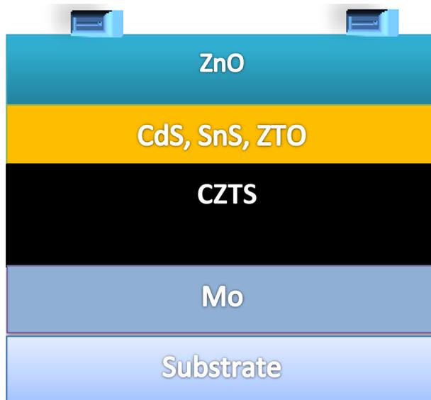
Fig. 1. Device structure of CZTS solar cell.
