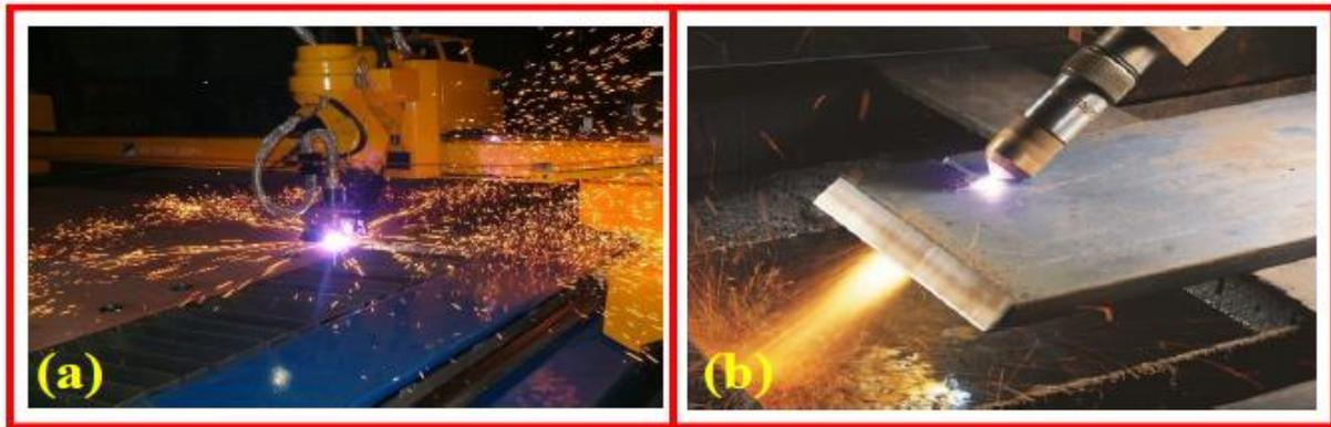
**Figure I.3 :** Exemples typiques industriels de torches de plasma: (a) Retro Systems LLC and (b) Hypertherm Inc [3].
